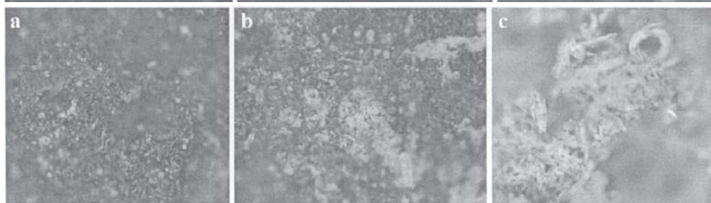
Fig. 3. OM images of surface structures on fragment S2: a and b - deposits of chemical compounds in the corrosion crust (100X); c - crystalline reformed microstructures in the corrosion crust (200X)
